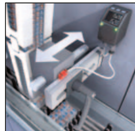
Monitored format adjustment on slide adjustment features with electronic position indicators.
