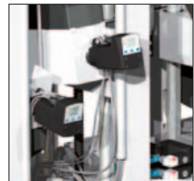
Full automation of spindles and machines by means of actuators.
